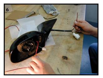
Pull the wire through the rubber sheath until six inches of wire remain exposed.
